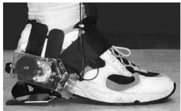
Fig. 5 - Rotating generator adapted in a shoe [14].
